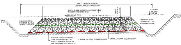
SECTION THROUGH NEW SITE ROAD CONSTRUCTION PHASE (CBR BETWEEN 1% and 2%)
