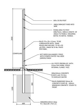
**Typical Palisade Fencing Details - Section** SCALE 1:50
