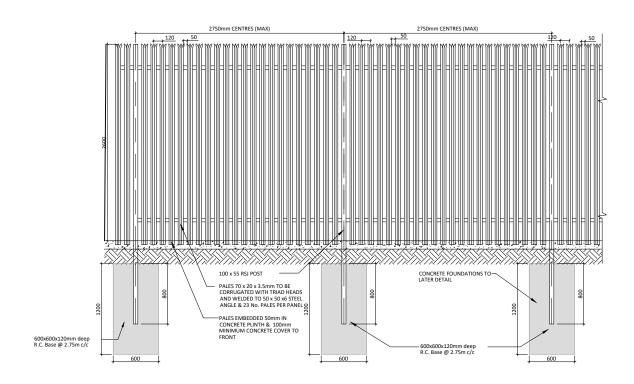
**Typical Palisade Fencing Details - Elevation** SCALE 1:50
